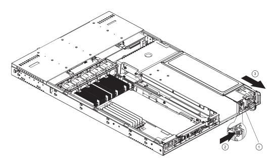
Figure 6-5. Removing/Replacing the Power Supply
